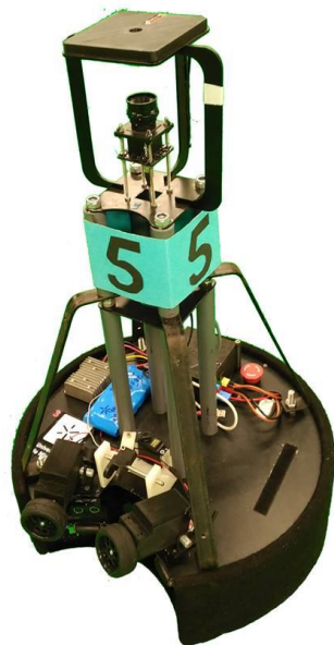
Fig.1. MinhoTeam's updated robotic platform, with the steel bars applied.
