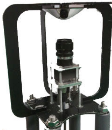
Fig.8 - Catadioptric vision system
